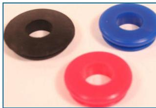
When using colored seals, put the proper color in each type of gladhand connector. Parking brake lines and fittings are red, while the service brakes are blue.
