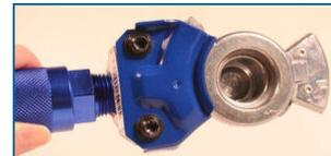
Before installing the new seal, use a clean rag to wipe the gladhand cavity clean. Gently remove any debris if applicable.
