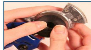
Install the new seal by positioning half of the seal in the air hole of the gladhand, aligning it squarely with the hole. Then press inward all around the seals surface to force the seal to lock into the groove all the way around. Rotate the seal several times once it's in place to make sure it is properly seated.
