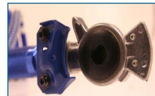
This is how a seal should look when installed properly.
