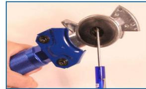
Easily remove the seal by gently prying them out with a screwdriver. Pay attention not to damage the gladhand surface.
