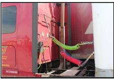
If your trailer is equipped with a quick release gladhand, be sure to service it as needed by removing the snap ring on the back of the head and checking condition of diaphragm on regular basis and wiping out the inside with a clean rag. Service kits are available if needed.
