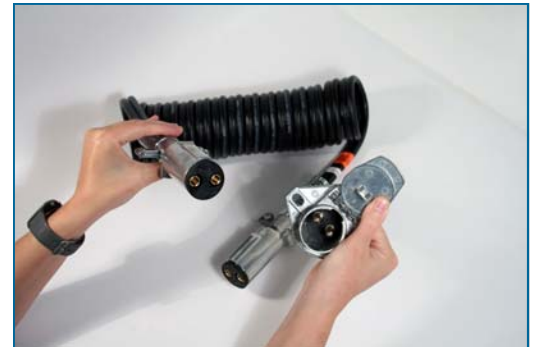
Dual pins in each plug and socket
