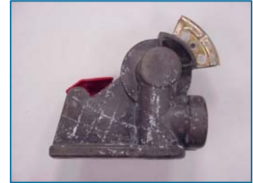
Anodized - minimal corrosion where scored
