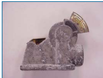
Standard - Heavy corrosion on entire body
