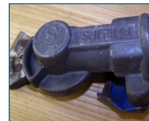
Anodized - Virtually no corrosion on the body
