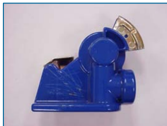
Powder Coated - Minimal corrosion where scored
