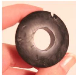
Broken edges and cracks indicate it's time to replace the gladhand seal
